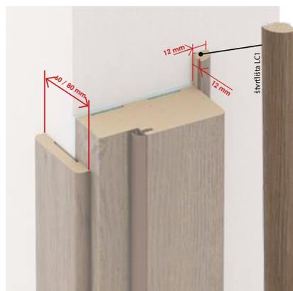
**KRYCÍ LIŠTA (LO1) MŮŽE BYT SPOLU SO ŠTVRŤVALČEKOM (LC1) POUŽITÁ PŘI BLOKOVÉ ZÁRUBNI, PŘI DVERÁCH SO ŠÍRKOU „60“–„90“.** PŘI DVERÁCH SO ŠÍRKOU „100“ JE POTREBNÉ OBJEDNAT SI KRYCÍ LIŠTU (LO2) ALEBO ZDVOJENÝ ŠTVRŤVALČEK (LC2).
