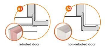
The edge of **rebated door** leaf is finished with a rebate (highlighted in red on the picture A1), which is placed on a door frame, when the door is closed. Door leaf produced in this way does not fit flush with a door frame.
